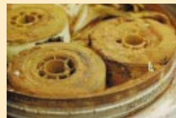
Loss of cinematographic heritage Decomposition of nitrate films Photo: Austrian Film Archives
