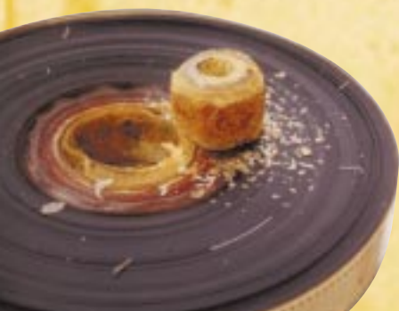
Loss of cinematographic heritage Decomposition of nitrate films Photo: Austrian Film Archives
